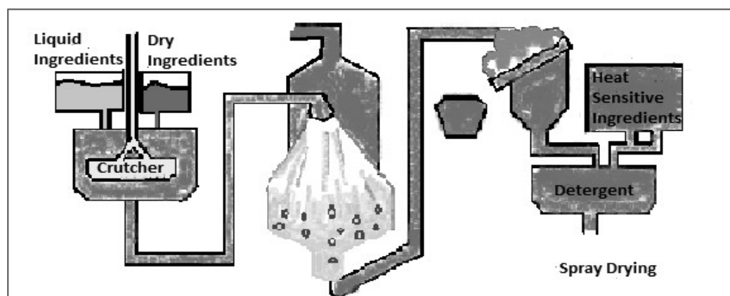
Figure 5: Diagram of spray drying
