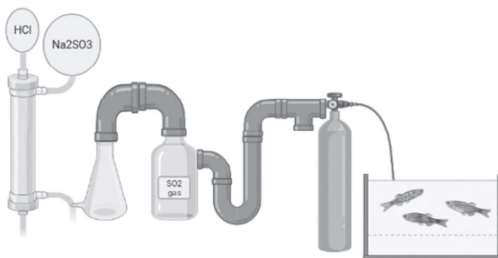
Figure 1: Experimental setup of production and exposure of gaseous sulphur dioxide to the aquatic environment
